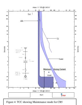
The addition and reduction of instantaneous pickup settings is just one way to reduce the hazard associated with low-voltage arcs. Light detecting relays or "Arc Flash Sensors" are devices which detect the light emitted by the arc fault. In the event of an arc, the light sensors send a trip signal to relay which in turn can trip the breaker in less than 2 cycles.
