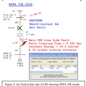
The results shown in Table 2 indicate that the incident energy released for a fault located at the line (incoming) side of the circuit breaker CB5 can be far more dangerous because of the longer operating time of the fuse. Figure 1 shows the Time Current Characteristic (TCC) of Fuse2 along with the expected fault clearing times for the minimum, maximum and arcing fault values.
