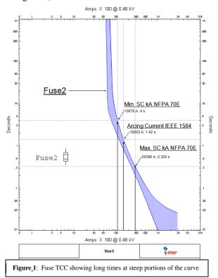
This article discusses methods available for calculating the incident energy released by an arc fault in low-voltage equipment. It also presents considerations which should be made to determine the worst-possible hazard associated with energized work at different locations of the equipment. In addition, it will cover methods to reduce the hazard level like maintenance mode settings and arc flash sensor relays.
