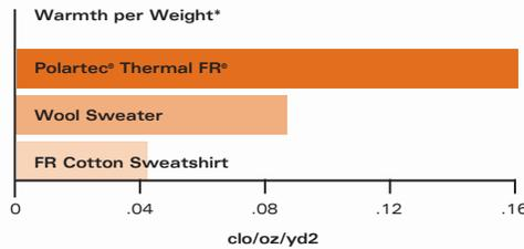
Thermal Transmittance/Insulation Test: The test is conducted according to ASTM D 1518. Insulation property is measured in clo values. The higher the clo value, the greater the insulation properties.
